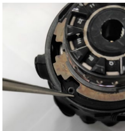
Figure 21: Push the hole of the glove around the boss for the screws
